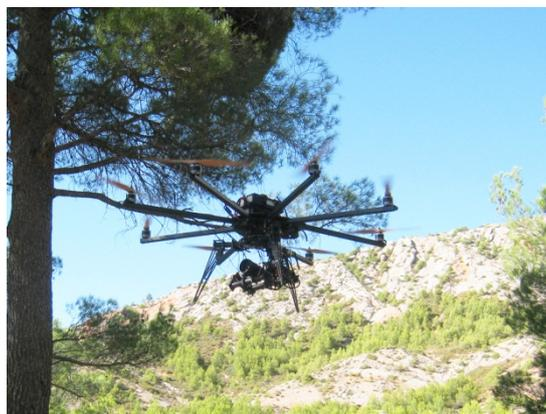
The *SmartAnalog* radio-controlled multicopter has eight propellers and a digital camera. The system can be operated by two people: a pilot and a camera operator equipped with a video viewfinder which displays the frame being shot in real time.
